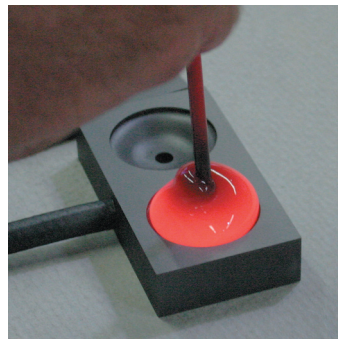
Photo 2 Press it into one of the two mold cavities, while holding the glass rod perpendicular to the mold. One cavity has a profile for making the top of the spinning top. The other cavity has a profile for the bottom. You can choose which you like best for each. However, the first half you make should be the top side of the spinning top, as this will save you steps.
